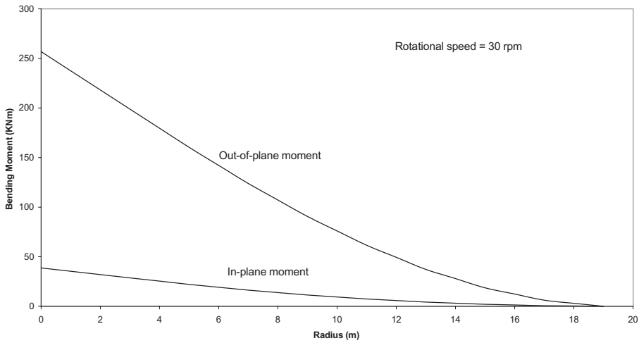
Figure 5.7 Blade In-plane and Out-of-plane Aerodynamic Bending Moment Distributions for Typical 40 m Diameter Stall-regulated Machine Operating in a Steady, Uniform 10 m/s Wind
