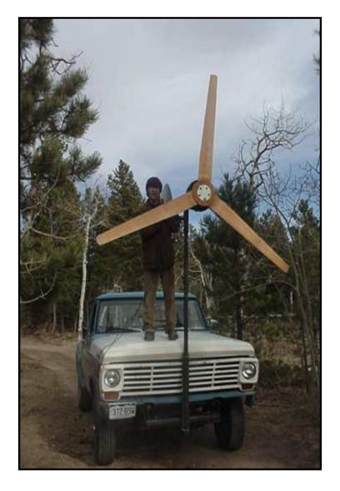
I bolted a piece of the same sign post we used to make the windmill onto the front of my '70 F250, and made some U clamps so that a 2" diameter pipe mast could be fitted. See in the picture above, I am wiring the alternator up for testing. This serves as an excellent test rig. On the passenger floor of the truck is a 12 volt battery, and enough meters on the seat to record whats going on! By watching the meters and my speedometer, and a still day, one can record good information about how the
