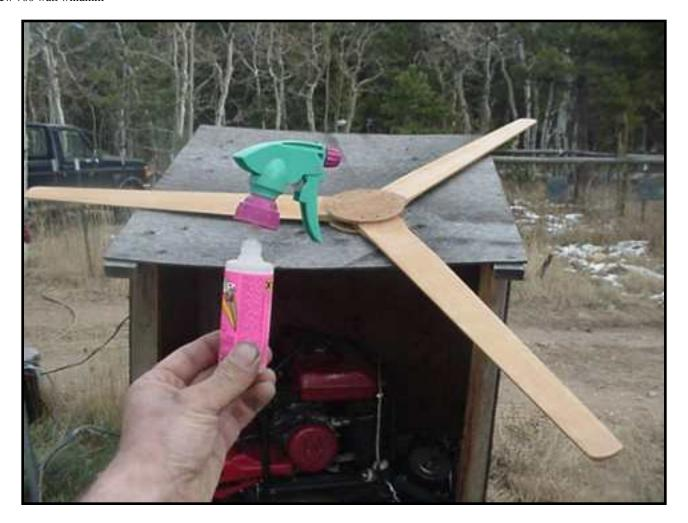
Once the epoxy dried, we finished the prop with "Super Glue" - from a spray bottle. Neat way to put a tough finish on wood, but horribly toxic and very expensive! (about \$50!). As it turned out, we smashed this prop and the next prop we simply finished with a thick coat of Linseed oil.
